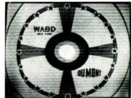
Fig. 5. Horizontal bar interference. Interference signals below 15,750 cps at the CRT cause this type of pattern.
