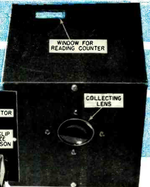
Fig. 1. External and internal views of the photoelectric counter. An X-25 phototransistor is the heart of the device.
