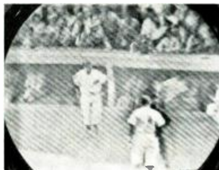
Fig. 4. Beat pattern caused by unmodulated r.f. signal above 15,750 cps. These lines can also appear vertically.
