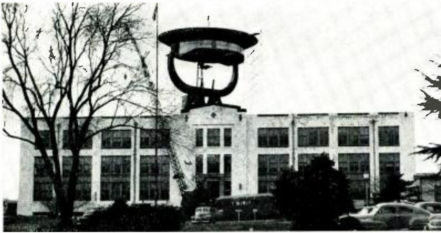
The 600-inch "radio telescope" installation at the Naval Research Laboratory which is being used to study radio "signals" from the sun, moon, and stars. Scientists use this research tool to extend man's knowledge of the universe and to assist in forecasting the conditions for radio communications work.
