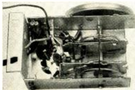
Fig. 8. Bottom view of the continuous-type u.h.f. tuner. Note the shielding.
