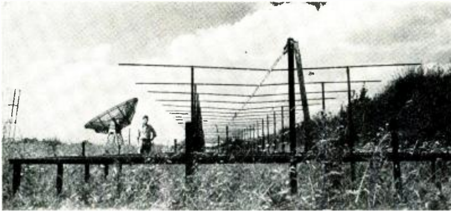
Fig. 2. Array of full-wave dipoles at 3.7 meters. This array is one-half of an interferometer for detecting radio stars. See text for full details.
