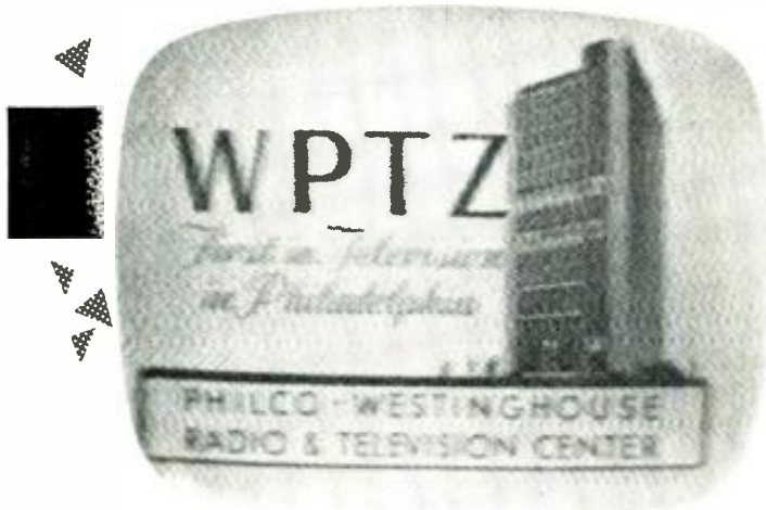
Fig. 1. Appearance of a 1.5 mc. FM beat on the face of a CRT. This pattern is not stationary but changes with the variations in sound carrier modulation.
