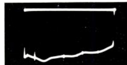
Fig. 6. Oscilloscope pattern produced by a 300-ohm line terminated by 330-ohm resistor.
